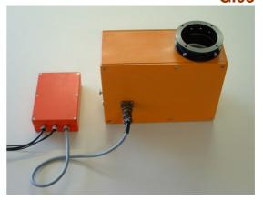
used as stand-alone measuring system providing an analogue output of 0-10 VDC resp. 0/4-20mA or they can be integrated into the META versatile QMS-9000 quality control system. Scanners or C-frames are available for fix-position or scanning measurements and controls.
