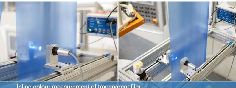
Inline colour measurement of transparent film
