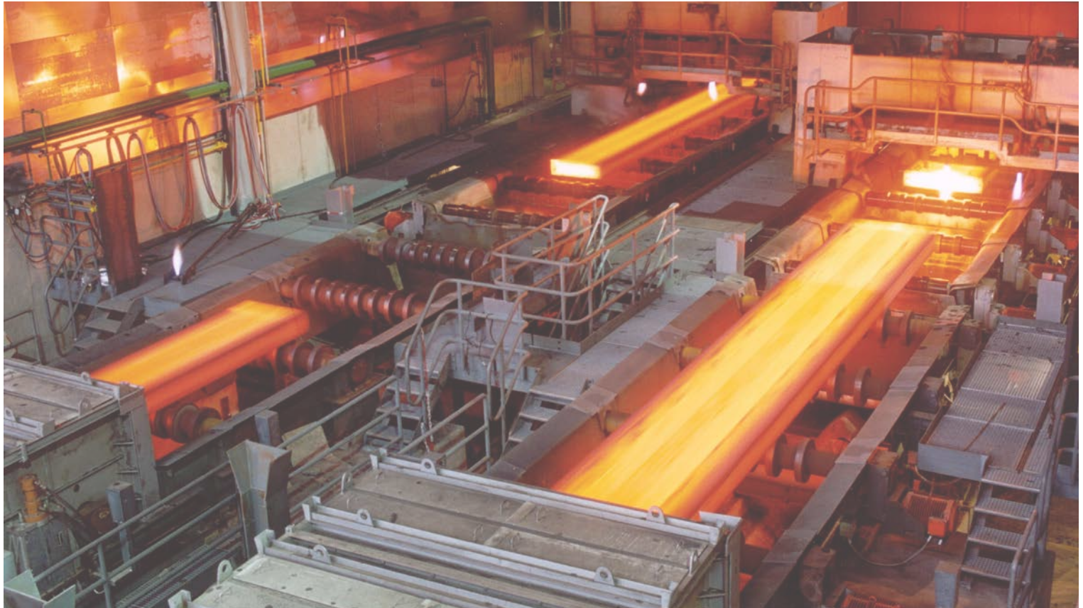
Temperature monitoring in hot rolling processes using the TIM M1
