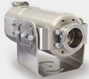
TM-J-CTL Cooling jacket (length 228mm, ø89mm) with adjustable mounting bracket TM-JAB-CTL; up to 315°C ambient temperature
