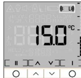
Fig. 22 Display measurement function low alarm
