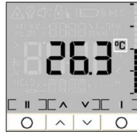
Fig. 28 Display measurement function temperature unit
