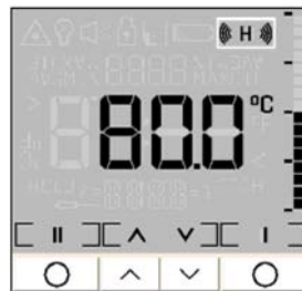
Fig. 20 Display measurement function high alarm
