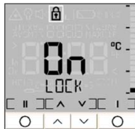
Fig. 24 Display measurement function long-term measurement (Lock Mode)
