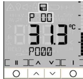
Fig. 40 Display storing measurement values
