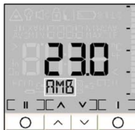
Fig. 35 Display measurement function ambient temperature compensation 1
