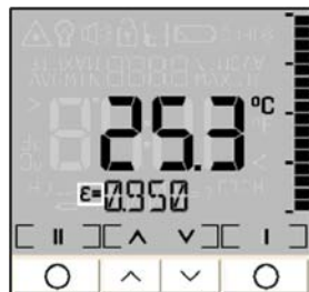
Fig. 18 Display measurement function emissivity setting
