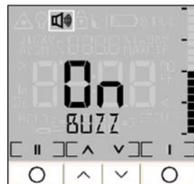
Fig. 30 Display measurement function buzzer
