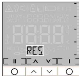
Fig. 38 Display measurement function reset
