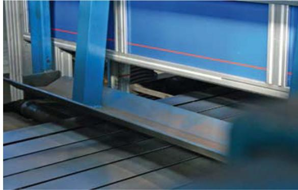
**Fig. 1:** Tilted strips in a slitter
