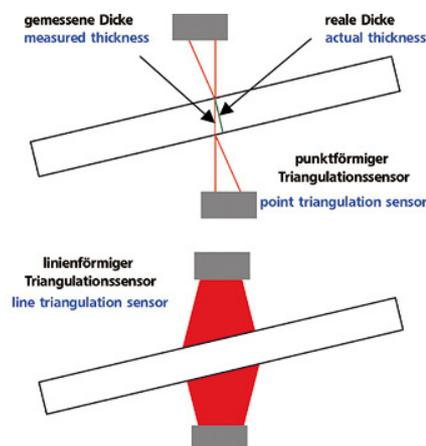
**Fig. 2:** Measuring error resulting from angle errors with point sensors
