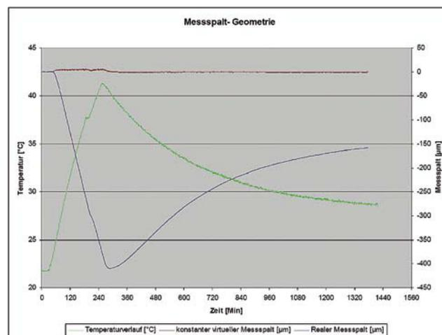
**Fig. 5:** Changes in stand-off distance as a result of thermal effects
