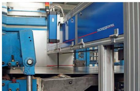
Fig. 6: Complete measurement with record of length using ASCOSpeed
