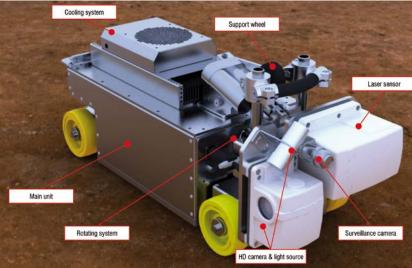
ROV (Remotely Operated Vehicle) for pipeline inspection
